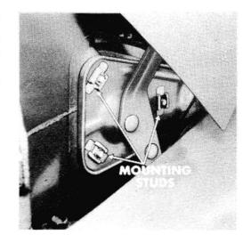
Slots at the rear edge of the hood are designed to permit side-to-side adjustment when the hood flares out too much or seats too far from the fenders.
