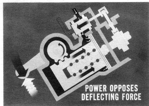
Fig. 7—Road shock reverses steering forces
