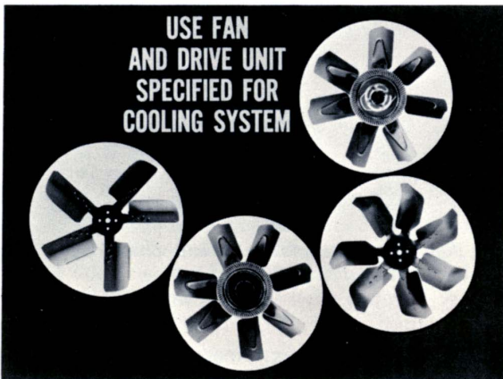
Fig. 21—Switching fans or drives can cause problems
