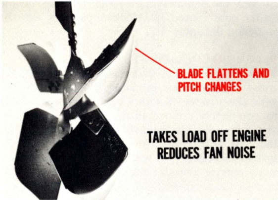
Fig. 20—Flex-blade fan speed is not limited
