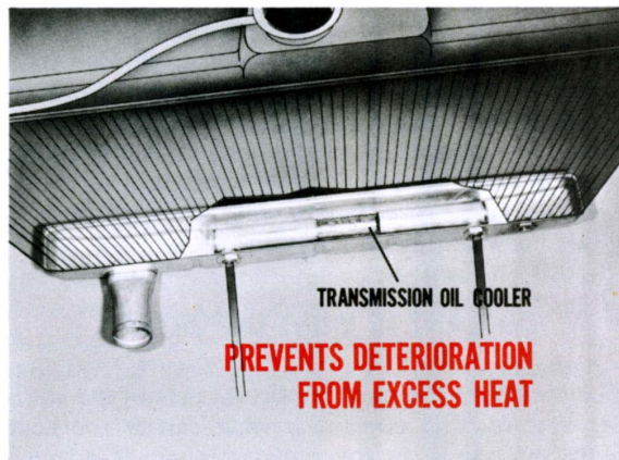
Fig. 6—Oil cooler is first place coolant picks up heat
