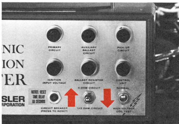
Fig. 33—Use toggle switch to check ballast resistor
