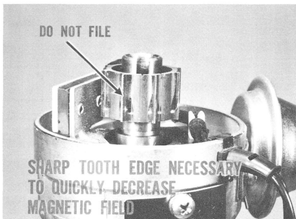
Fig. 15—Reluctor teeth are sharp
