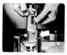
you'll have a lot of nice grinding compound resting on that top ring. Then, when you push the piston out, that grinding material will make some nice deep scratches on the cylinder wall, and you're in for trouble.
