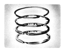
control rings are similar to the standard production rings. The difference in the Oil Saver ring set over the production ring set is that the Oil Saver combination uses a spring steel expander behind the second compression ring and the two oil control rings. Those expanders give a little more ring tension against the cylinder wall and insure that the rings will follow the taper of the wall closely.
