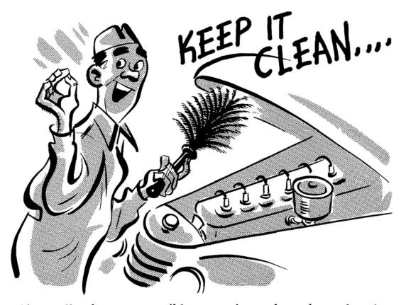
Above all, take every possible precaution to keep the engine clean while you're working on it. Dirt is the worst enemy of an engine. If it gets into the cylinders or the intake valve ports, it is sure to cause trouble.
