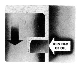
against the cylinder wall. So the piston goes down on its power stroke with the full face of each compression ring flat against the cylinder wall.
