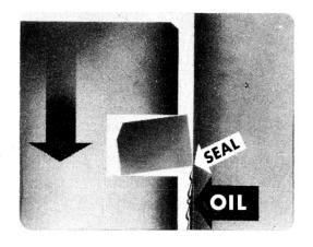
engine will blow blue smoke out of the tail pipe like nobody's business! When the ring is compressed and installed in the bore it twists, so just the lower outer corner contacts the cylinder wall.
