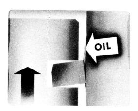
during the intake stroke. But the oil can't get up . . . those edges are wiping it down . . . cleaning the wall.
