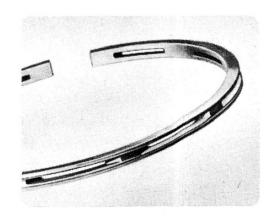
Any army backs up its first line of defense with a second line . . . that's why we back up the first (or bottom) oil control ring with a second oil control ring. It is necessary for some oil to get up to the compression rings, but not too much. Therefore, the second oil ring takes care of the excess oil that gets past the first ring, permitting only the right amount to get up on the compression rings.
