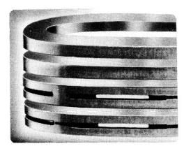
The rings in this illustration had a hard time. They're scuffed and worn. This is what happens when the driver has a lead foot. Those vertical scuff marks are made by particles of metal which have seized to the cylinder wall and then scratched the rings as they rotated on the piston.
