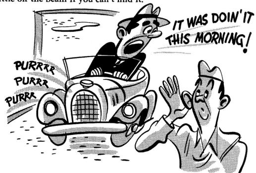
It's the kind of piston slap that occurs only when the engine is cold. It's a piston slap, all right—but it's usually caused by a tight fitting piston pin. And you can hear it with the engine idling—the engine doesn't have to be pulling. By the time the engine warms up the piston expands and frees up on the pin, so the knock goes away.
