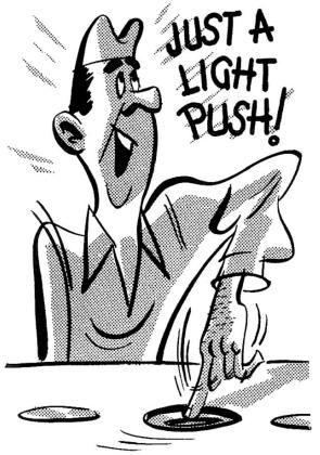
You see, the cam ground piston has two high sides—the thrust faces. You should fit the piston in the cylinder so it will pass through the bore with a light push of the hand . . . you can stop it anywhere in the bore and it will barely hold itself in place without falling through of its own weight. Just a nice, even, light push all the way through the cylinder.
