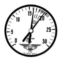
Worn Guides. When the vacuum gauge needle vibrates rapidly while the engine is idling you can be pretty sure that the trouble is caused by worn intake valve stem guides. This is because air is being drawn in between the valve stem and the guide, reducing the vacuum in that cylinder.
