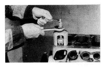
Now, the new insert can't conduct the valve heat to the water jacket unless it makes a good tight fit in the counterbore. So, if the insert is loose in the block, counterbore the block and install a ten-thousandths oversize insert.
