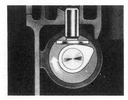
Then the quieting ramp comes into action again for the last four thousandths of valve movement (assuming that tappet clearance is ten thousandths), and eases the valve down onto its seat gently, so that it won't make noise.
