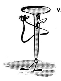
VALVES. The valves have a simple job to do, but it's a mighty important job! They have to open and close passages to the combustion chamber, to let fuel in and exhaust gas out. And they have to seal the combustion chamber tightly to prevent loss of pressure. That's why the valves are ground to make a perfect seal with their seats, and that's why they're made of special heat-resistant steels.
