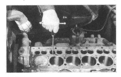
When you're replacing guides, be sure to drive them in to the exact depth specified for the model you're working on. You see, it's important to get the guide in to the proper depth in the block. You can scale off the specified depth and mark it on the driver, so you'll know how far down to drive the guide.
