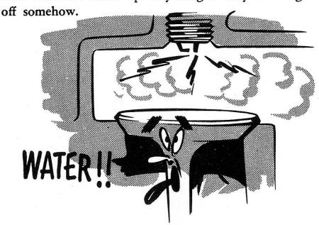
Of course, the answer is that the valves pass on their heat to their seats, which in turn are cooled by the water flowing through the water jacket. The exhaust valve seats get extra cooling from cool water circulated around the seats by the water distributor tube. The intake valves receive additional cooling from the incoming fuel mixture. But the important point is this: the valves have to do most of their cooling during the time they're in contact with their seats.
