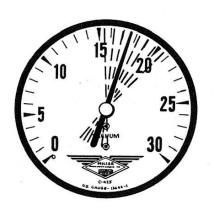
Weak Springs. You can spot weak or broken valve springs by speeding the engine up to about two thousand r.p.m. If the springs are weak, the vacuum gauge needle will fluctuate rapidly between about twelve and twenty-four inches of vacuum. Of course, if a spring is broken, the needle will fluctuate rapidly every time that valve attempts to close.
