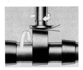
whenever it's lifted. The rotating action helps to neutralize the effects of wear, because it prevents wear from being concentrated on any one spot on the tappet face or on the tappet body.
