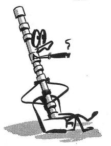
in the valve family because it controls the movement of the tappets and the valves. The cams are positioned around the camshaft in such a way as to open and close the valves in the right order. To synchronize the action of the valves with the movement of the pistons, the camshaft is connected to the crankshaft by the timing chain.
