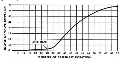
The area of the cam face that's under the tappet during the first thirty degrees of rotation is the "quieting ramp." Actually,
