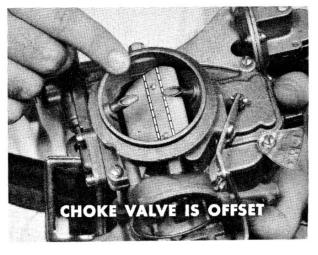
the incoming air tends to force the valve open against the tension of the thermostatic coil. The result is the proper positioning of the choke valve, according to engine speed and load conditions.
