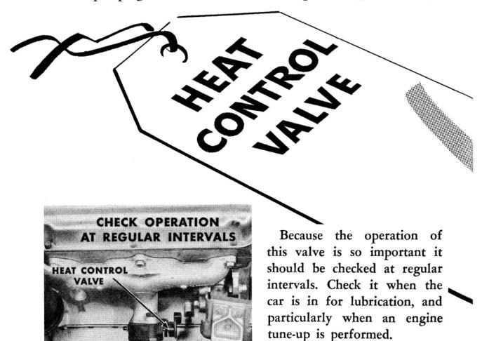
To check the operation of the manifold heat control valve, first quickly accelerate the engine wide open, then quickly release the throttle. This action should cause the exhaust gases to exert a force on the valve which causes the shaft, with its counterweight, to respond by rotating, then returning to normal position.
