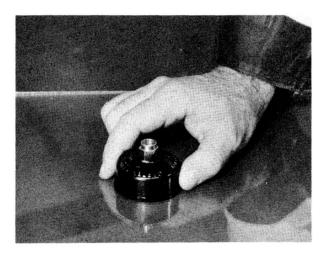
If the housing appears to be in good condition, check it for being warped by trying to rock it on a surface plate, or a pane of glass. Make sure that you remove the heat retainer plate assembly before you make this warp test.
