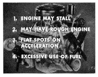
When the exhaust gases are not properly directed to the hot-spot chamber in the intake manifold several conditions may result: The engine may stall. You will have a rough engine. You will have flat spots on acceleration, and the owner will talk about excessive
