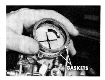
While you've got the choke housing off and the heat plate removed, clean all parts of the choke mechanism with solvent and blow dry. This will clean out all possible points of restriction.
