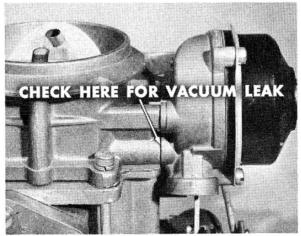
There's one other place where you could get a vacuum leak on carburetors where the metal choke housing is separate from the air horn.
