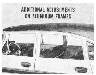
Rear Door Adjustment. On cars with the aluminum frame doors, you start your door adjustments with the *rear door*. You'd make hinge adjustments to fit the door to the opening, and then check the fit and seal above the belt line.
