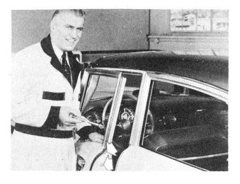
As you did on the rear door, if one edge fits well, but the other edge is out of line, loosen just the bolts on that edge. Then readjust that edge and tighten the bolts you loosened, along with the bolt at the division bar.
