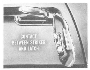
door lifts slightly so you hardly notice the lift. There should be firm contact between the striker and latch to prevent rattles when the car is driven over rough roads. Be sure to keep the striker in a level plane. If you tip it so it enters the latch at an angle, the door will be hard to open and close.
