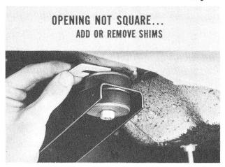
shims at the body bolts. If you find that you do have to add or remove shims, loosen all the body bolts on the side you're working on. And, after adding shims at any bolt, shim the adjacent bolts if you find it's needed to keep the body supported evenly on the frame.
