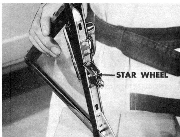
Fig. 6 — Vent-wing-pivot tension adjustment
