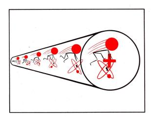
Before the advent of the electron theory, it was assumed that an electric current flowed from positive to negative. Today, we know for sure that electrons do flow from negative to positive. In present-day troubleshooting, don't worry about the direction of electron and current flow. Connect the battery correctly and the direction of current flow will take care of itself.
