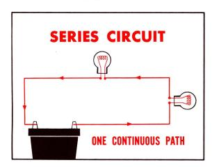
Since there is only one continuous path for current flow in a series circuit, all of the current must pass through each resistance in the circuit. The amount of current flowing depends on the total resistance of the circuit and the amount of voltage applied. Since current is the rate of electron flow, the current in amperes will be the same at all places in the
