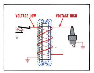
Since there are thousands of turns of fine wire in the secondary winding, the induced voltage is very high. High enough to jump a spark plug gap. Since there are far fewer turns in the primary winding, the voltage induced is relatively low.
