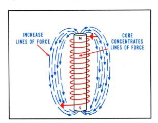
The addition of an iron core to an electromagnet greatly increases its magnetic strength. That's because the iron core offers very little "magnetic resistance" (reluctance) as compared to an "air core".
