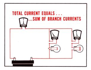
The total resistance of a parallel circuit is always less than any one resistance in the circuit. This is explained by the fact that the total opposition to current flow offered by the parallel resistance units is less than that of any one of the resistance units. In other words, each of two parallel paths will allow more current to flow than either of the individual paths or circuits.
