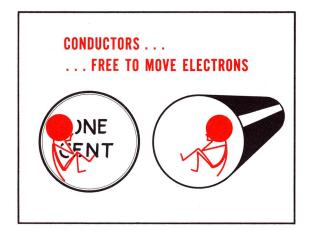
There are just as many free electrons in a copper penny as there are in a copper wire made of the same copper alloy. In other words, free electrons are always present in a conductor regardless of whether or not that conductor is ever used in an electrical circuit.
