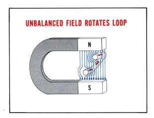
After the loop rotates one-quarter turn, the conductor is in the weakest part of the field. In addition, the unbalanced field condition at each side of the loop is no longer trying to rotate the conductor. Instead, it is trying to push the conductor outward . . . away from the field. The loop will stop rotating.
