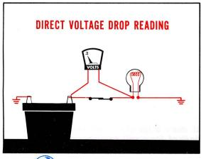
Direct Voltage Drop Measurement. A direct voltage drop reading can be made by connecting the voltmeter across a part of the circuit. When a voltmeter is connected across a part of the circuit it registers voltage drop across that part of the circuit, not voltage available.
