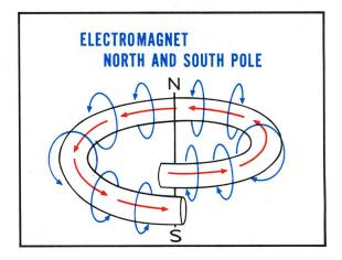
If more loops are added to form a coil, the lines of force will pass through the center of the coil, out the end and reenter at the other end. This produces the same field pattern as a bar magnet.
