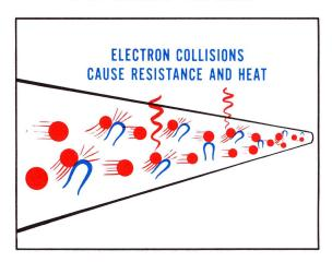
The number of collisions between the electrons and atoms also increases when the number of electrons flowing is increased. This accounts for the fact that a conductor carrying a current is heated to some extent and is heated more when current flow is increased.
