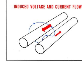
Now, if two wires are side by side and current is flowing in one wire, the lines of force from this wire will spread out and cut across the second wire. What happens when lines of force cut across a wire? Now in an alternator stator, alternating current is flowing in all windings. Lines of force spread out from each wire and cut across the adjacent wire. This induces a voltage which opposes the original voltage and current flow. This is commonly called inductive reactance.
