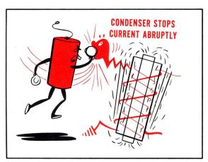
In addition to preventing arcing, the condenser stops current flow in the primary windings very abruptly. This in turn speeds up the collapse of the magnetic field, increasing the speed at which the lines of force cut the secondary windings. Increasing the speed of the collapsing magnetic lines increases the voltage induced in the secondary. You can see how important condenser action is to maximum ignition voltage and point life.
