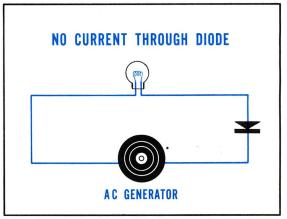
When the output current from an alternating current generator tries to change direction, no current can flow through the rectifier. For all practical purposes, the circuit is disconnected when current flow tries to reverse.
