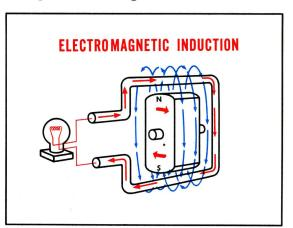
loop of wire, the magnetic lines of force will cut across the wire or conductor. The moving lines of force cutting across the conductor cause the free electrons in the conductor to start moving. A voltage has been electromagnetically *induced* in the conductor.
