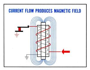
. . . without any *mechanical* movement. This is the basic principle used in an ignition coil. When two coils are close together, electrical energy is transferred from one coil to the other through a magnetic coupling. This is called "mutual induction" and is the action that occurs in an ignition coil.
