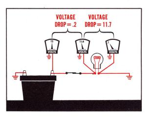
not exactly the same at any two points in a circuit because a voltage drop always occurs when current is moved through a resistance.
