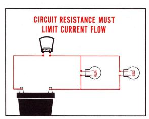
An ammeter is always connected directly into a circuit in series . . . it becomes part of the circuit. The circuit resistance must be high enough to limit current flow to an amount less than the maximum capacity or rating of the ammeter. In other words, the resistance
