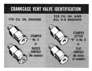
six-cylinder engine. A different size valve is used for the 225-cubic-inch six-cylinder engine and all V-8 engines. These valves must not be interchanged.
