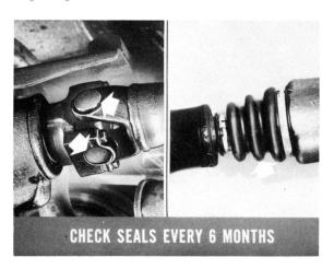
Inspection requirements: The universal joint seals should be inspected every six months. The joints should not be disassembled or relubricated unless there is evidence of leakage or seal damage.
