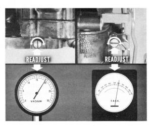
Readjust mixture and speed: Very carefully readjust mixture until you again get the highest, steady vacuum reading. If idle speed increases again, readjust it.
