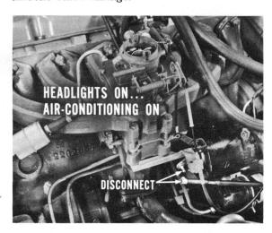
Vacuum gauge and tachometer: Since high manifold vacuum is the best indication of a good idle mixture, use a vacuum gauge. Don't trust your ears to tell you when the exhaust "sounds like the right mixture". Don't trust your eyes or your sense of touch to accurately detect engine smoothness. The correct idle mixture at specified idle speed is most important. Don't guess at idle speed . . . use a reliable tachometer.
