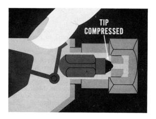
Invert the air horn so that only the weight of the float is seating the needle when you check float level. If you have to adjust the float level, remove the float. If you try to bend the float level tab when the float is in place, you'll probably compress the needle tip. After the job's all buttoned up and ready for delivery, the tip will regain its shape and the float level will be low.
