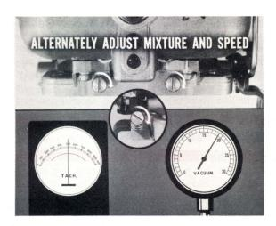
mixture changes the speed. Always go back and readjust the idle mixture after readjusting idle speed to see if you can get a still higher, steady vacuum reading.
