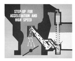
Sustained stumble or hesitation: If you get full power when you step on the gas but performance fizzles out as soon as the engine has used up the extra shot of fuel from the accelerator pump, the trouble is probably in the step-up system. Don't confuse this trouble with inadequate fuel supply which is covered a bit later.
