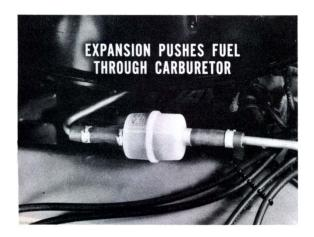
hot-spots. In addition, they have been repositioned so that they are tipped at a 45-degree angle or positioned upright. Here's the reason for repositioning the filters.
