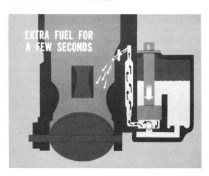
Momentary stumble: If you get a momentary stumble on acceleration from any speed when you step on the gas, the trouble is probably in the accelerator pump. If the engine picks up the load and accelerates normally after that first momentary hesitation, the step-up system is probably okay.
