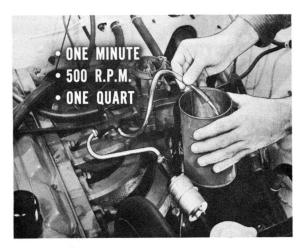
If fuel delivery through the filter is less than one quart in one minute, repeat the test without the filter in the line. If fuel delivery is okay, the trouble was in the filter. If fuel delivery is still low, the fuel pump, the fuel lines or possibly a restriction at the tank inlet is causing the trouble. The fuel pump pressure
