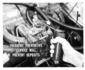
A treatment of carburetor cleaner at least every six months will greatly retard the accumulation of deposits. In some cases, it's a good idea to administer this preventive service every two months . . . when the engine oil is changed. You don't have to disassemble the carburetor . . . just use a small squirt can to get cleaner into the critical areas.
