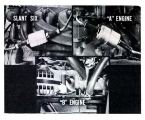
If you want to know where to put the filter on an early-production or past-model car, just take a look at a late-production job having the same engine and equipment. Get out your flaring tool and tube-bending set and you can make a new line in less time than it takes some owners to start a flooded engine.
