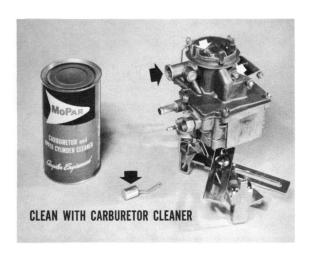
piston and clean both the piston and the cylinder with carburetor cleaner. Also soak the air horn in carburetor cleaner to loosen and remove deposits from the choke shaft bearing areas. The importance of cleaning deposits from the choke shaft bearings is frequently overlooked. Current production carburetors have been modified to reduce the shaft bearing area and minimize choke shaft sticking.
