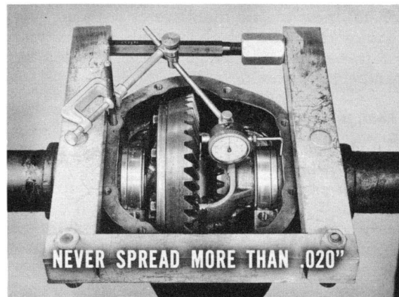
Fig. 4—Spreading the carrier housing
