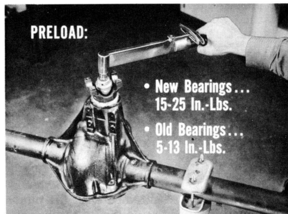
Fig. 10—Testing pinion bearing preload
