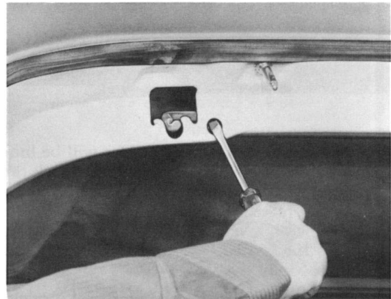
Fig. 8—Turn screw to adjust torsion bar
