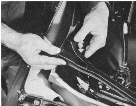
Fig. 11—Check weatherstrip for distortion
