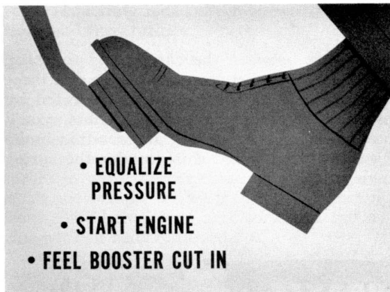
Fig. 21—Test power brake operation
