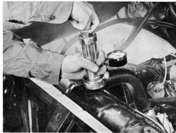
Fig. 5—Pressure-test the cooling system
