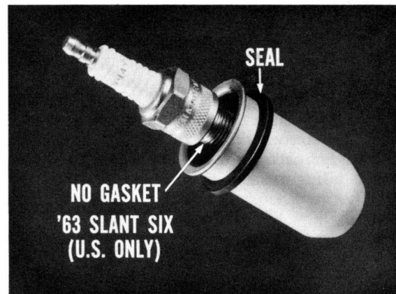
Fig. 14—Replace seal when servicing plugs
