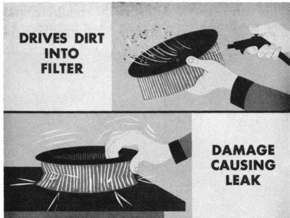
Fig. 9—Improper filter cleaning techniques
