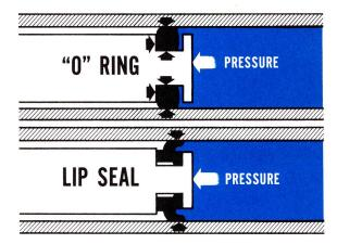
"O" rings are used effectively where motion is limited to seal closely fitted parts. They seal in both directions and take up little space. When the mating parts are assembled together, the "O" ring is squeezed at the inside and outside diameters. Pressure on either side of the "O" ring forces it against the side of its groove providing a positive seal on three sides.
