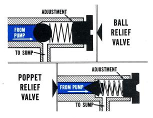
A relief valve is like a check valve in construction, except that it has a heavier spring to hold it seated against pressure. An adjusting screw can be turned in or out to vary spring tension, and thereby vary the pressure at which the valve relieves. Most simple check valves use a ball to seal against pressure, but a coneshaped poppet also is common.
