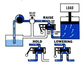
In a third position, all three ports are open to each other. Pump delivery is bypassed to the reservoir along with the fluid under the hoist cylinder and gravity lowers the load.
