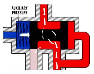
The auxiliary pressure can be applied to plugs at the valve spool ends or to differential areas in the valve grooves.
