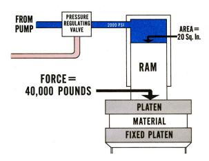
Fluid is pumped into the other end of the ram and a valve in the line regulates the pressure that can be developed. If the pressure-apply area at the end of the ram is 20 square inches and the pressure developed is 2000 psi, the total force at the platen is 40,000 pounds or 20 tons.
