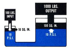
So, if we're able to take the ten psi we just created and apply it to a piston with a 100-square-inch area, we can exert a total force of ten times 100 or 1000 pounds. Force is multiplied—with a 100-pound input we obtain a 1000-pound output, ten times as much. And in fact, input force can be multiplied 100 to one, or even 1000 to one just by increasing the size of the output piston.
