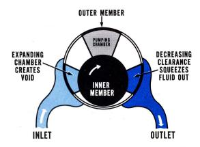
The size of the chamber continues to increase until rotation carries it past the inlet to the point of maximum clearance. For a few degrees of travel here, the chamber neither increases nor decreases.
