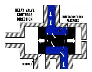
They are like a traffic cop, telling the fluid "stop here" or "now you can go". They are held in one position by spring force. When pressure opposing the spring rises high enough, the valve shifts and connects ports. Auxiliary pressures can be applied to relay valves, too, but the valves are designed so they don't meter—they just open and close.
