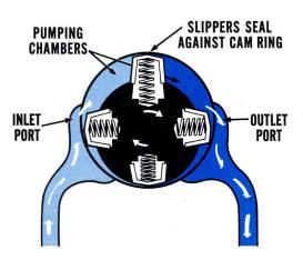
Pumping chambers are formed between two slippers, which seal against the ring. The chambers are carried from the inlet to the outlet by the rotor turning.
