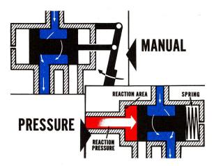
resolved into force by multiplying the pressure and reaction area. The valve will always move in the direction of the greater force.
