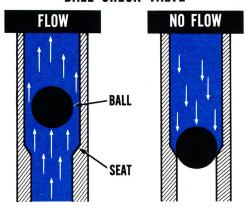
In the TorqueFlite valve body, there are several ball check valves with two seats connected to different pressure chambers. In this type of valve, the ball is seated by the higher pressure and blocks the lower pressure.
