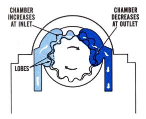
the lobes are meshing again, decreasing the chamber size and squeezing the fluid out into the system. The inlet is sealed from the outlet by the close clearance between the lobe tips at the point of maximum displacement.
