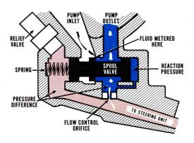
orifice is ported to the spring end of the valve and assists the spring in holding the valve closed.
