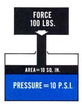
The pressure created in the fluid is equal to the force applied, divided by the piston area. If the force is 100 pounds and the piston area is ten square inches, pressure equals ten psi. According to Pascal's law, this pressure of ten psi is equal everywhere in the trapped fluid:
