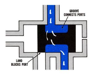
A spool valve is cylindrically shaped, with two or more lands and with annular grooves between the lands. The valve is closely fitted to a round bore and slides in the bore on a pressurized film of fluid. Fluid passages are open or closed to each other, depending on the valve land positions.
