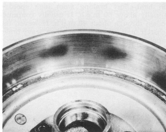
Fig. 8 — "Incipient" heat spot
