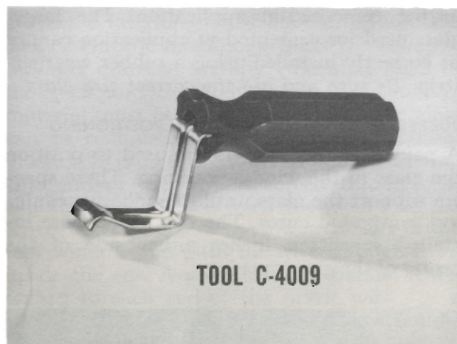
Fig. 8—New windshield and rear window removing tool
