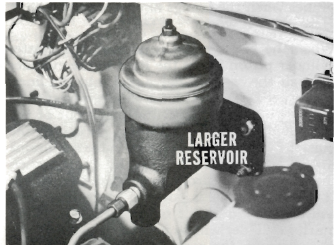
Fig. 12—A bigger fluid supply
