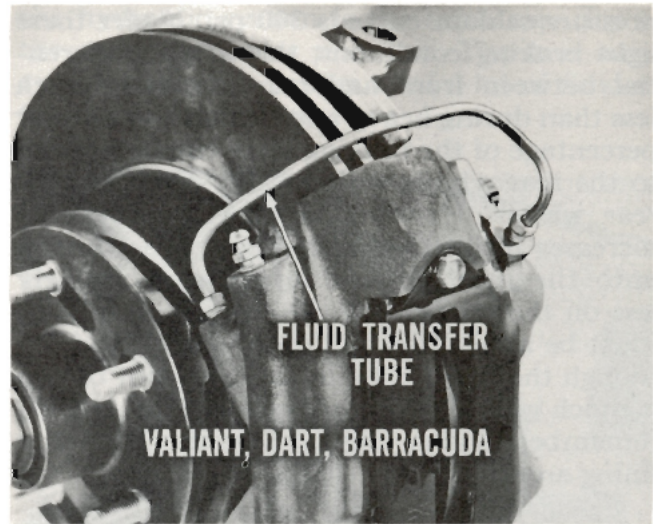
Fig. 17—Tube supplies outer caliper half
