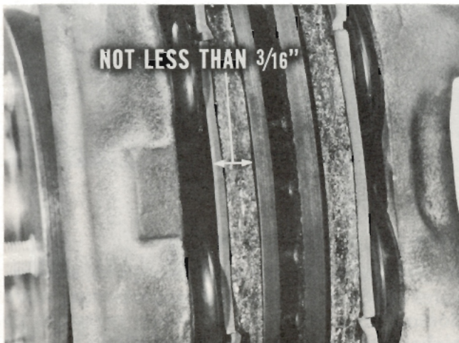
Fig. 18—Time to replace linings
