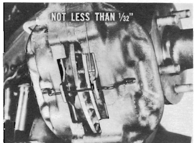
Fig. 29—Maximum lining wear
