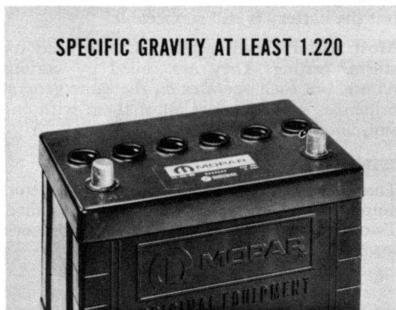
Fig. 14 — Load test needs \frac{3}{4} charge or better
