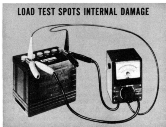
Fig. 15 — Below 9.5 volts calls for replacement
