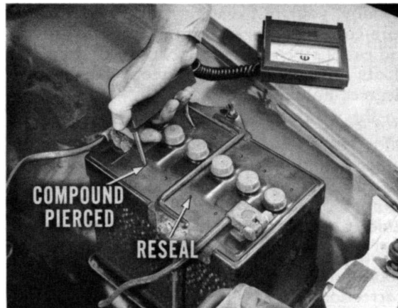
Fig. 10 — Reseal against surface leakage
