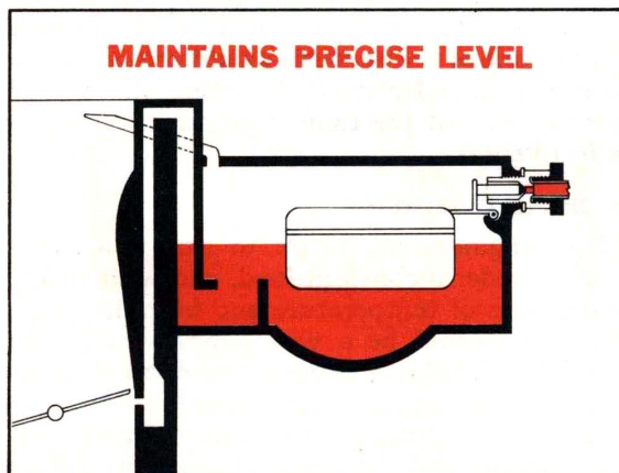
Fig. 8—Float bowl is storage tank
