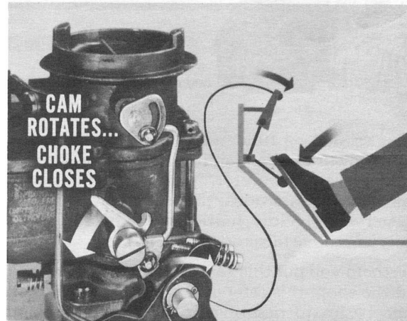
Fig. 3—Pedal releases fast-idle cam
