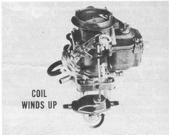
Fig. 4—Thermostatic coil closes choke
