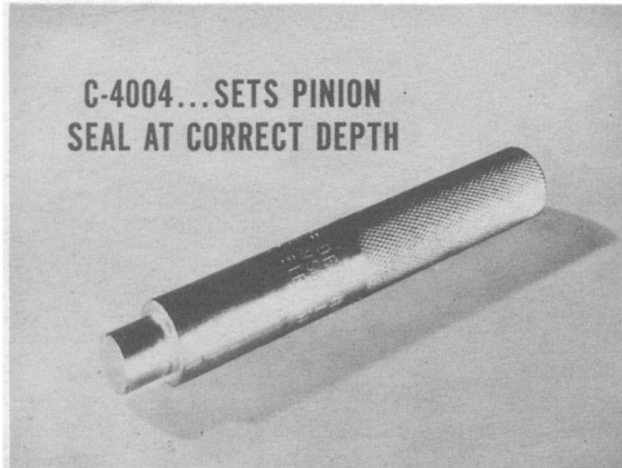
Fig. 22—Essential installing tool
