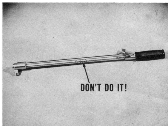
Fig. 37—Stamping or etching weakens beam
