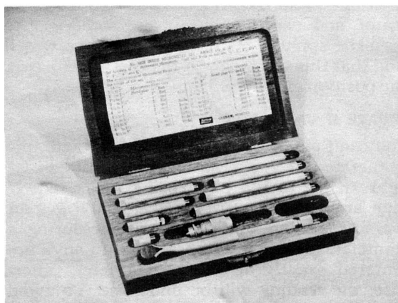
Fig. 11—Set of inside micrometers
