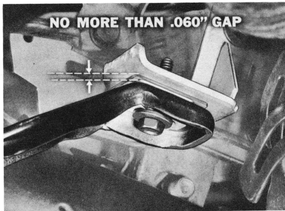
Fig. 18—Shim to avoid binding
