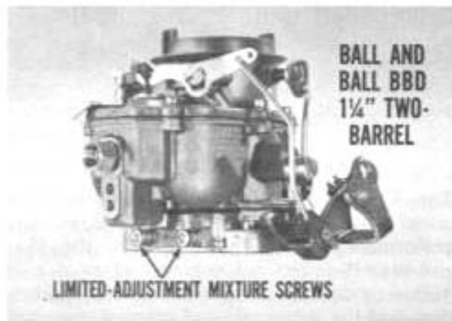
Fig. 6—Mixture screws are not removable
