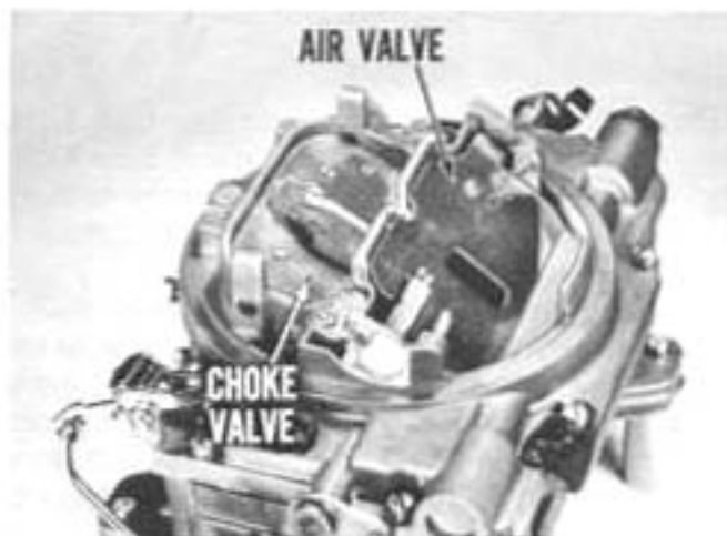
Fig. 8—Air valve looks like choke valve
