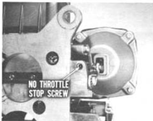
Fig. 28—Stop screw setting is eliminated
