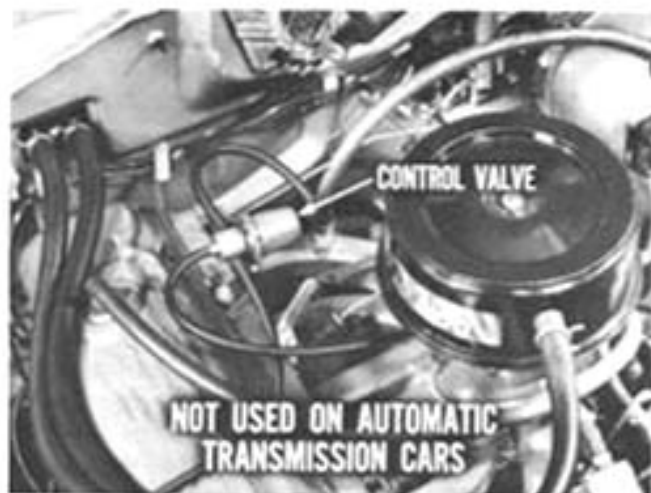
Fig. 1—Control valve needed only on some cars
