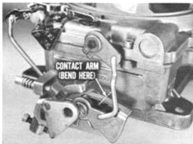
Fig. 20—Arm has larger contact surface
