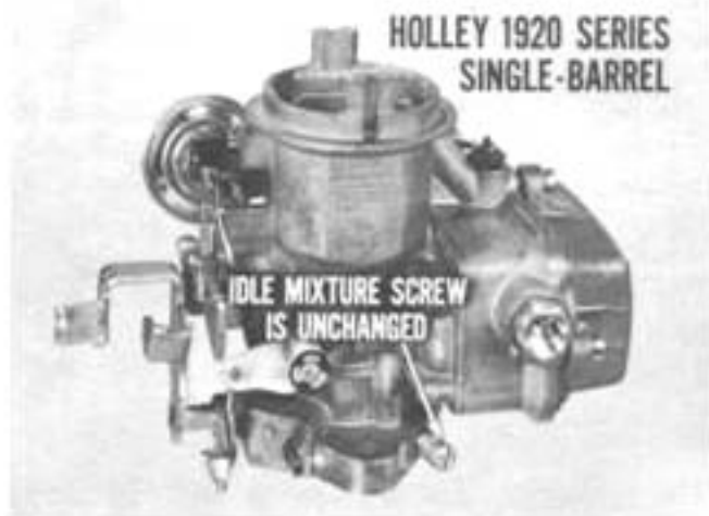
Fig. 4—Mixture screw can be removed
