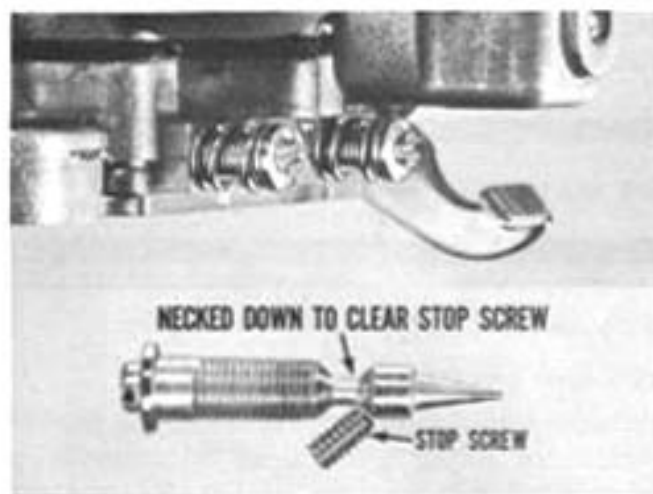
Fig. 32—Stop screw prevents mixture screw removal
