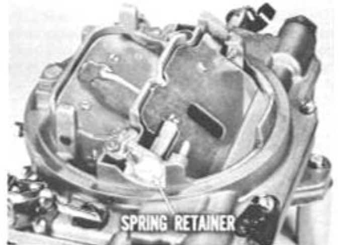
Fig. 12—Retainer setting adjusts spring
