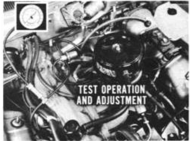
Fig. 35—Control valve drops distributor vacuum
