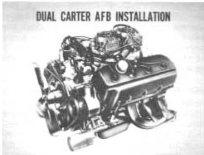
Fig. 29—Both carburetors have idle systems
