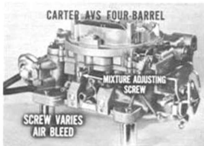
Fig. 13—Single screw adjusts idle mixture
