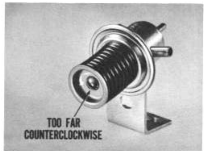
Fig. 36—Open valve keeps timing advanced
