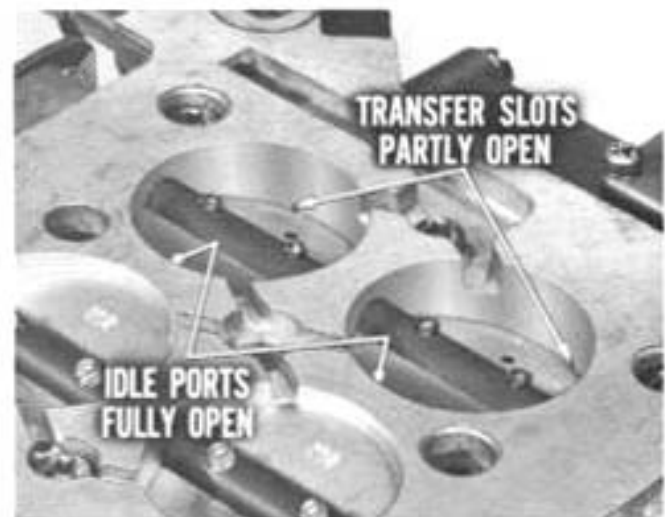
Fig. 25—Ports are on opposite sides of bores
