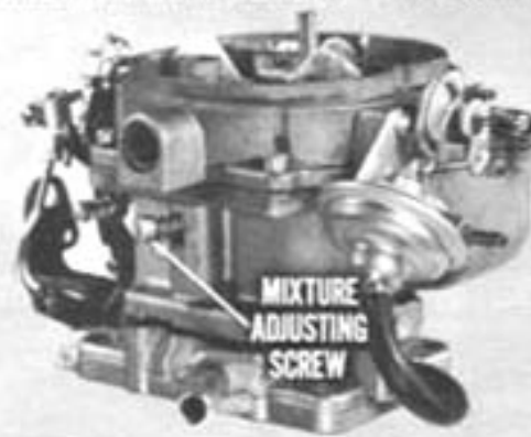
Fig. 21—Single screw controls both barrels
