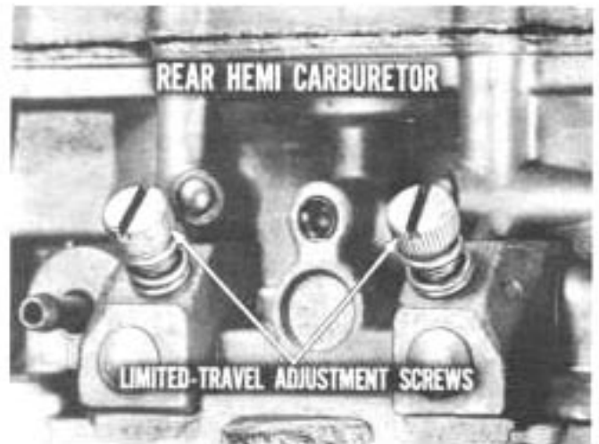
Fig. 31—Mixture screws cannot be removed
