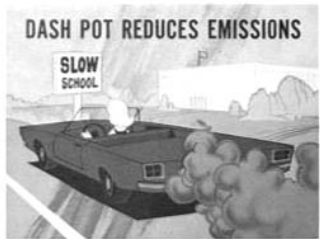
Fig. 2—Dash pot slows throttle closing
