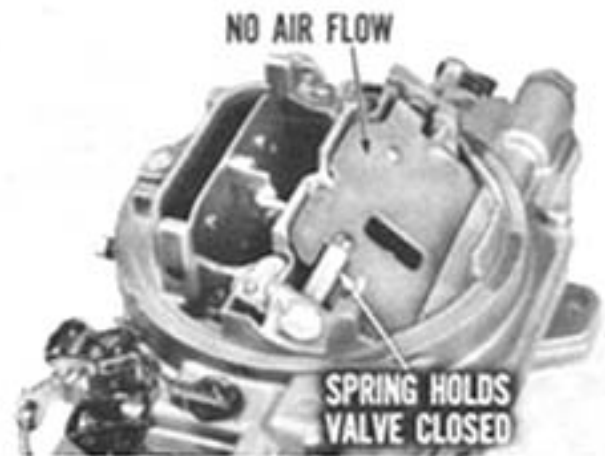
Fig. 9—Valve is opened by air flow
