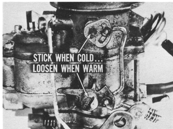
Fig. 10—Gum-type deposits cause choke and cam to stick
