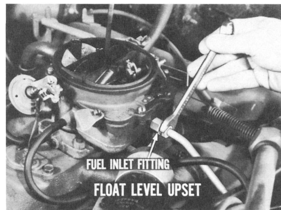
Fig. 35—This can upset carburetor float level
