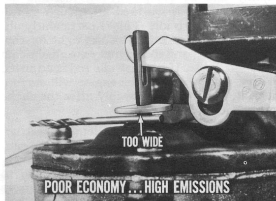
Fig. 16—Correct bowl vent opening is important
