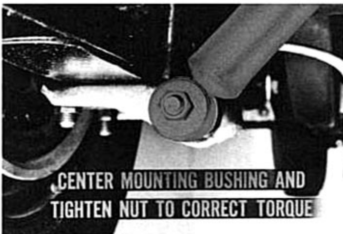
Fig. 31—Center bushings in their normal load position
