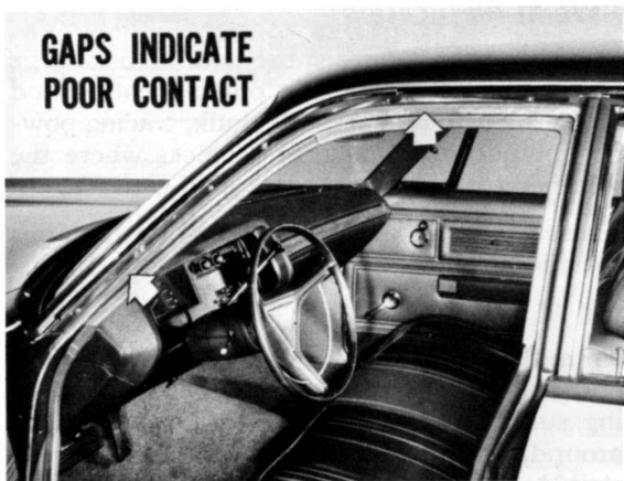
Fig. 15—Inspect chalk print all around
