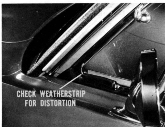
Fig. 30—Weatherstrip pucker leaks air
