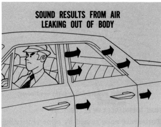
Fig. 4—Interior pressure forces air out
