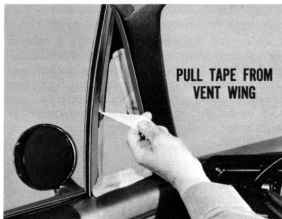
Fig. 25—Leaks show up as tape is removed
