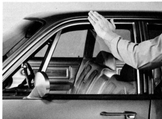
Fig. 11—Move hand around door edges
