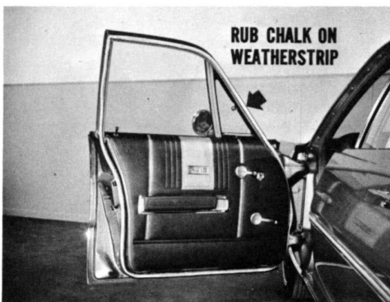
Fig. 13—Chalk transfers to door opening
