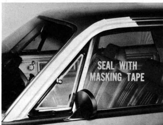
Fig. 23—Close off space for test
