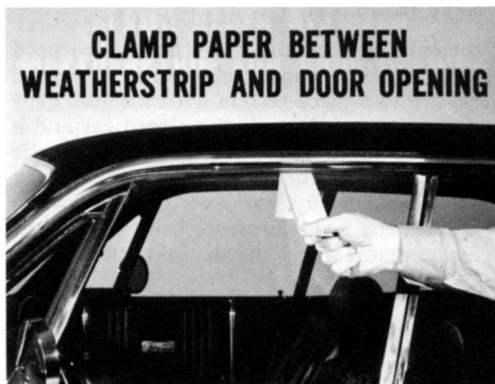
Fig. 16—Strip should pull with slight resistance
