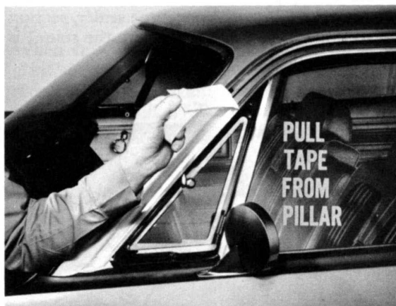
Fig. 24—Expose pillar area to air stream
