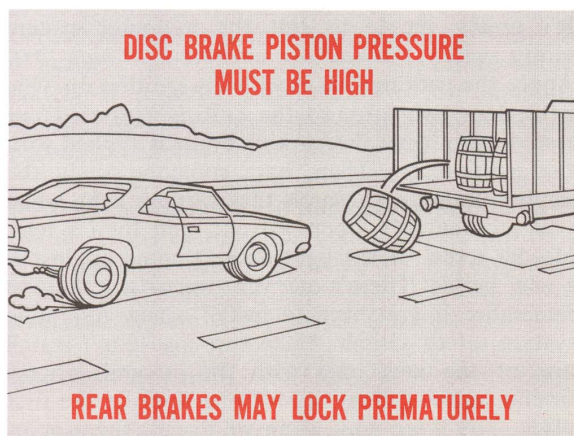
Fig. 20—Tire traction reduced by weight shift
