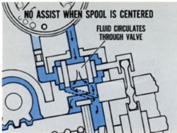
Fig. 11—Valve in balanced condition
