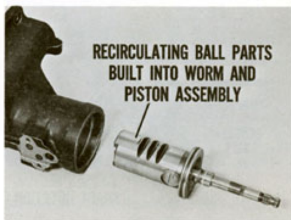
Fig. 2—Gear housing acts as cylinder
