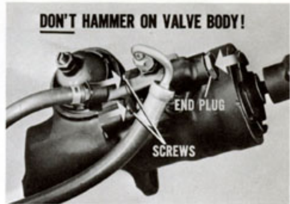
Fig. 41—Tap on end plug or body screws
