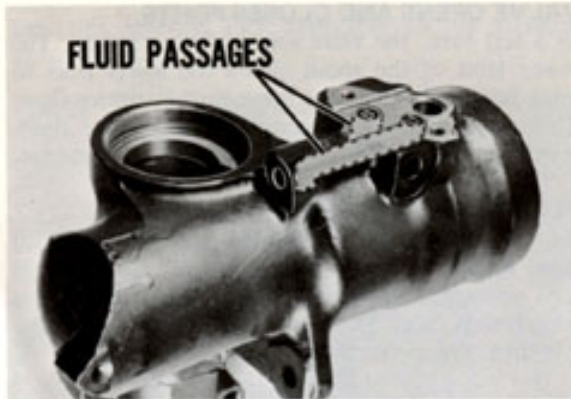
Fig. 7—Passages lead to power chambers
