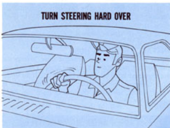
Fig. 37—Jolting may restore valve function
