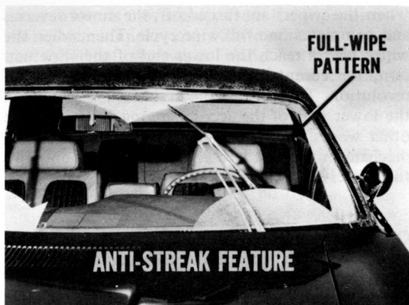
Fig. 17—Wiper completes full wipe pattern
