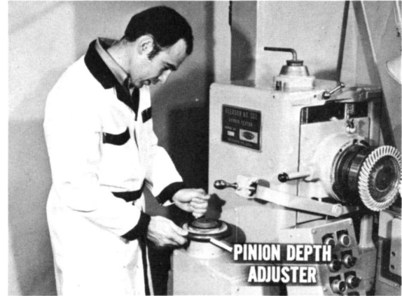
Fig. 18—Machine operator determines spacer thickness
