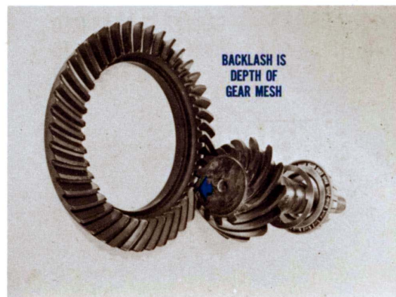
Fig. 36—Wrong backlash is another cause of noise
