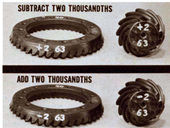
Fig. 34—Spacer size changes opposite of markings
