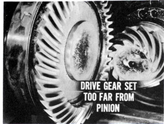
Fig. 38—Sharp line in pattern at top edge
