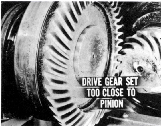
Fig. 37—Pattern has sharp line at root of tooth
