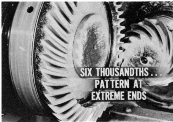
Fig. 27—Pattern heavy at toe and root
