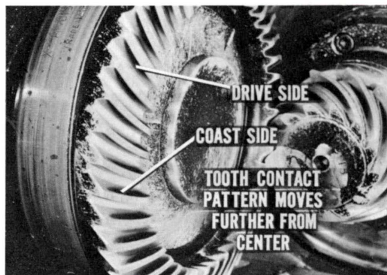
Fig. 22—Pattern moves farther on both sides of gear
