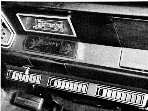
Fig. 2—The air-conditioning controls and air outlets
